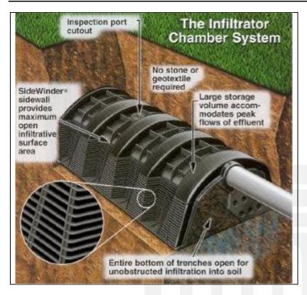
Figure 8 - Septic Infiltration Chamber
